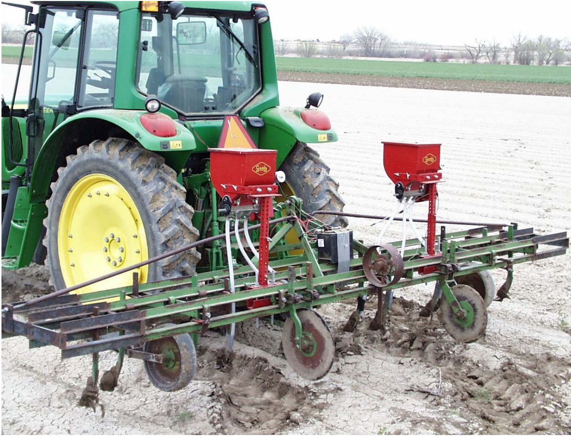
Figure 2. Chisel-slot opener of type used to apply Agri-Blend with Gandy boxes feeding the six inside rows. The outer untreated rows are used for comparison to the inside treated rows.
