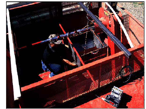
Lot Robinson operating the weigh bin inside the grain tank of a commercial combine.
