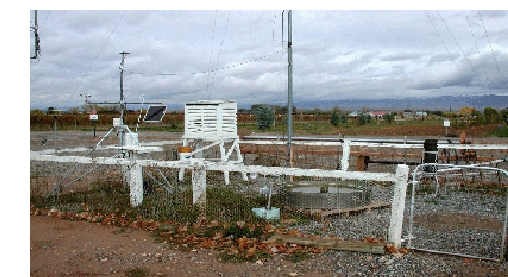
Manual (shelter) and electronic datalogger weather station (tripod unit at left) used to collect weather at Western Colorado Research Center-Orchard Mesa
