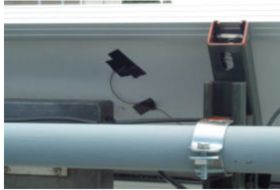
Figure 4: Thermocouple attached to the backside of panel
