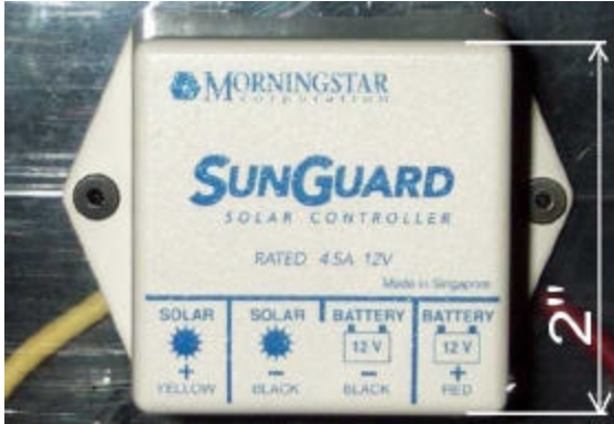
Figure 3: Moringstar Charge Controller (5 cm square)
