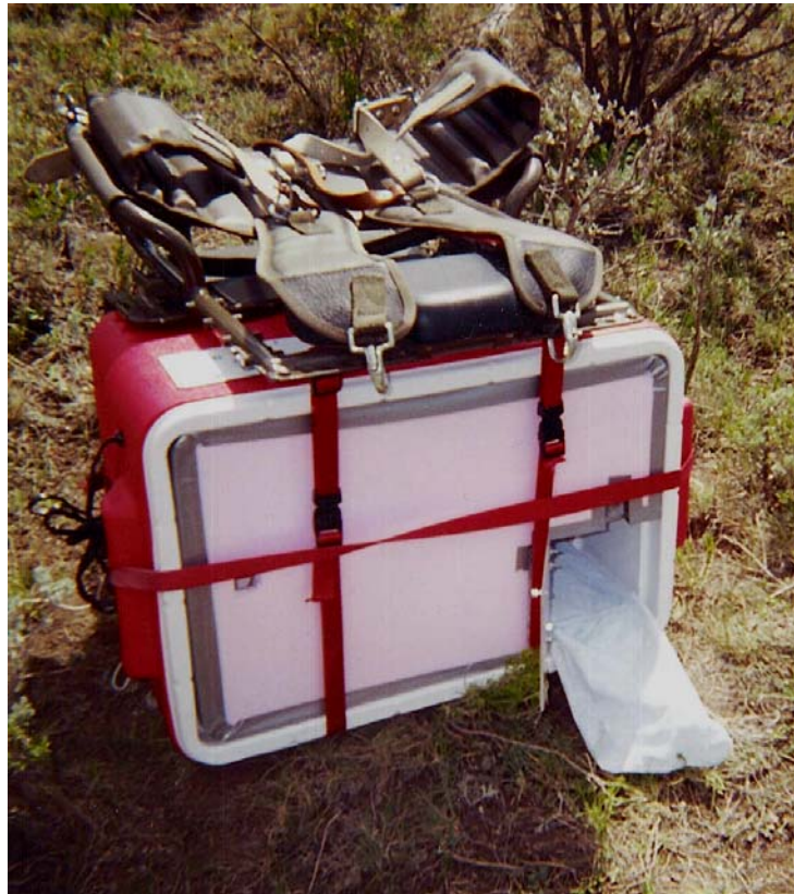
Fig. 1.1: Portable brooder used during field exposures of human-imprinted sage-grouse chicks to brood areas of Middle Park and Moffat Count, Colorado in 2002 and 2003, respectively. Note the entrance at the lower right and the backpack, on top, for transport.
