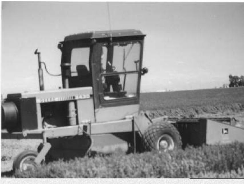
Fig. 2. The John Deere 3430 crimper/swather with electronic weigh box added to weigh each individual plot.
