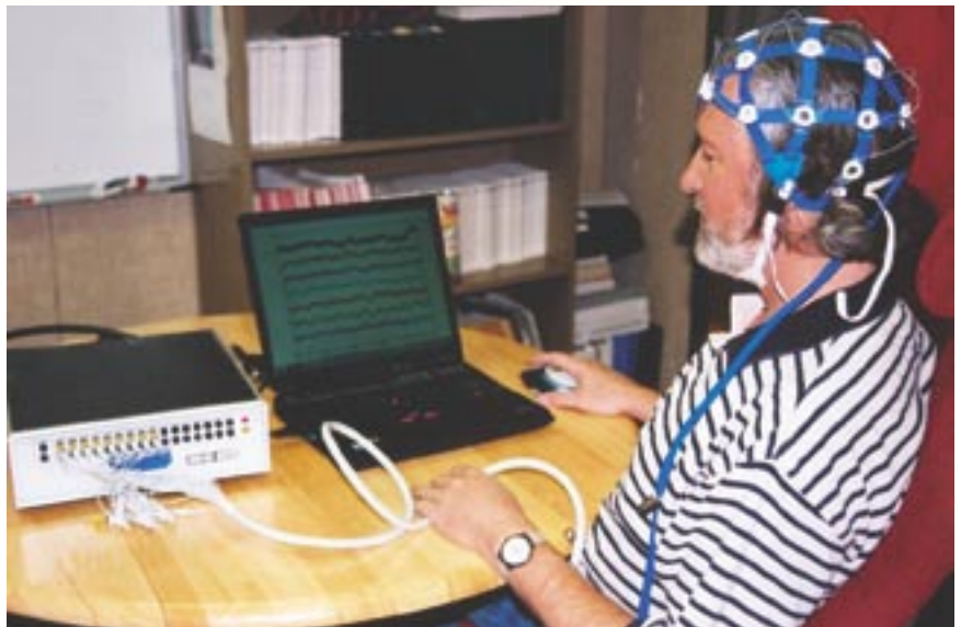
Chuck Anderson uses an electrode cap, EEG amplifier, and laptop computer to track brainwaves.
