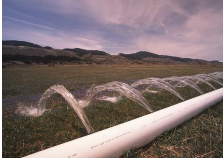
Figure 5 - Gated Pipe – the use of a sock at each gate will reduce erosion.
